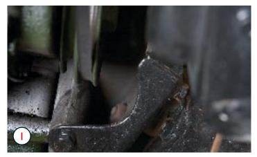
Symptoms: Knocking noise during engine acceleration/deceleration Diagnosis: Deteriorated engine steady mounts
