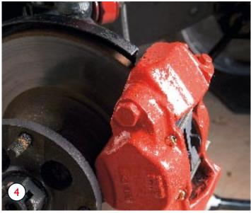
mptoms: Car pulling to one side when braking Diagnosis: Brake dust build-up
