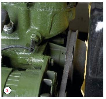
Symptoms: Squealing noise on start up Diagnosis: Faulty water pump
