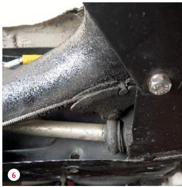
Symptom: Handbrake not holding Diagnosis: Seized handbrake cable
