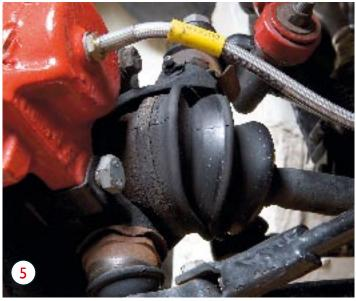
**Symptoms:** Knocking noise from the front with the steering on lock Diagnosis: Worn CV joint bearings
